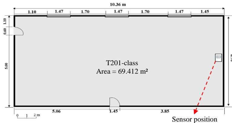
Fig. 3. T201-class dimensions and smart sensor position.
