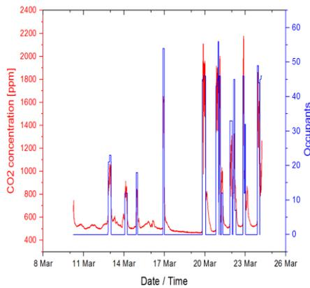
**Fig. 4.** CO<sub>2</sub>-concentrations and occupancy rate during the first period of IAQ measurement.
