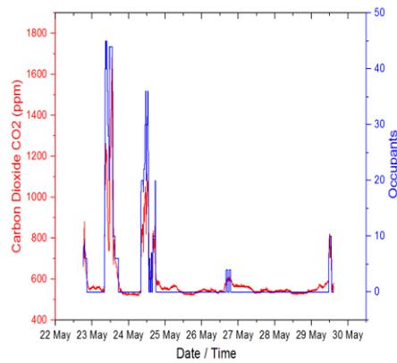
**Fig. 5.** CO<sub>2</sub>-concentrations and occupancy rate during the second period of IAQ measurement.
