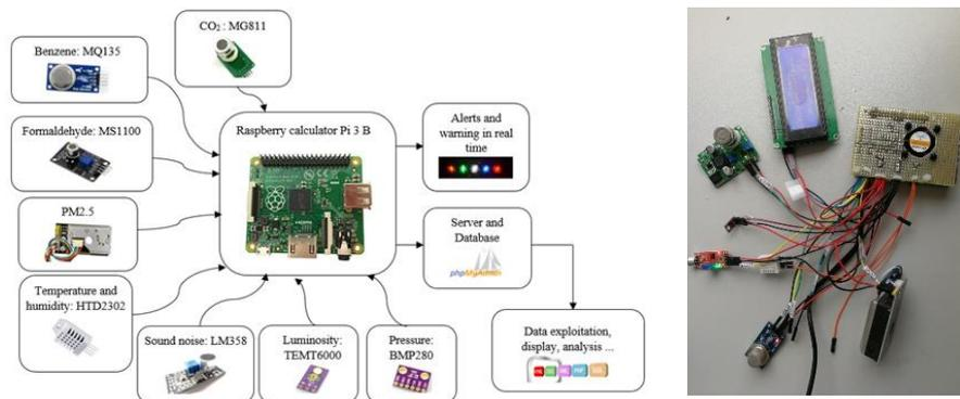
**Fig. 13.** Development of the smart IAQ sensor and comfort parameters (CO<sub>2</sub>, VOCs, CO, Formaldehyde, Benzene, PM2.5, humidity, temperature, noise and brightness).
