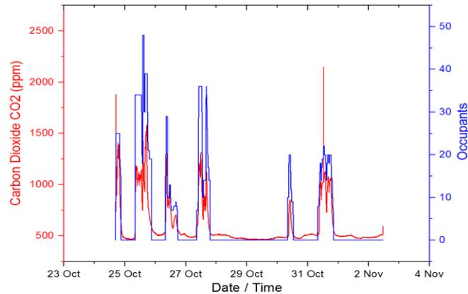
**Fig. 6.** CO<sub>2</sub>-concentrations and occupancy rate during the third IAQ measurement period.
