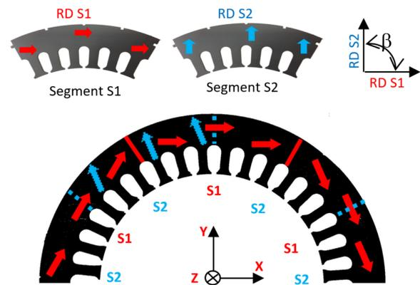
Figure 1: Implementation of shifted segments in SMC
