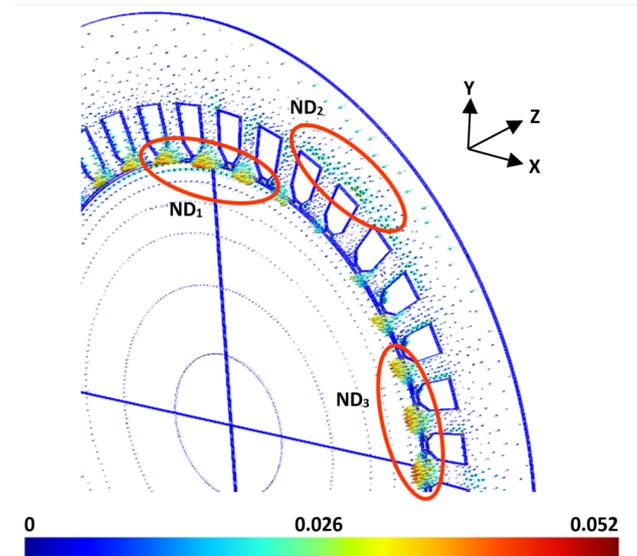
Figure 7: Distribution of  $b$  in the interlaminar air-gap
