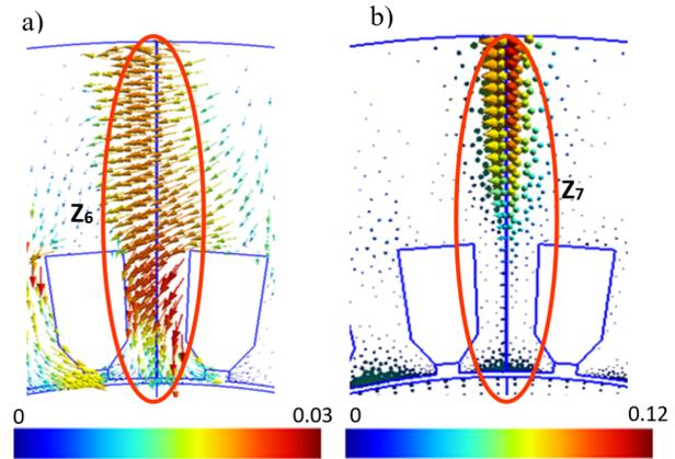
**Figure 9:** Joining zone of the two segments. Distribution of  $b$  in: a) the plane of the sheet and b) the interlaminar air-gap
