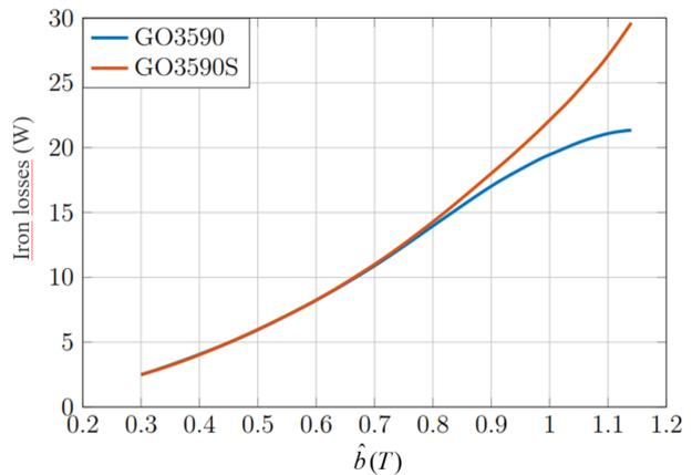
**Figure 4:** Comparisons of iron losses values
