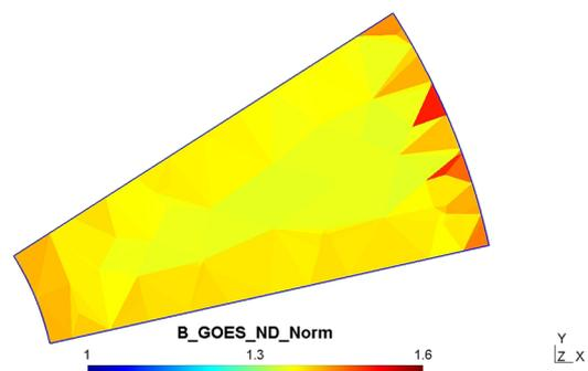
**Figure 12:** GOES rotor tooth induction levels (configuration # 2).
