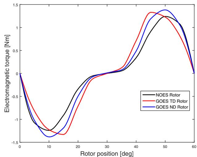
Figure 9: Torque variation with rotor position.
