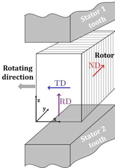
Figure 2: GOES rotor configuration #1.
