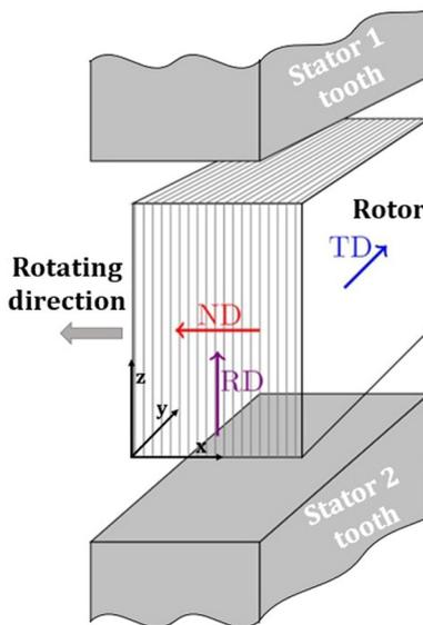
Figure 3: GOES rotor configuration #2.
