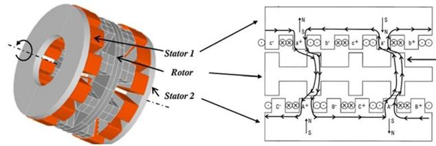
Figure 1: AFSRM and flux path.
