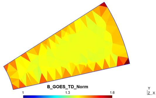
**Figure 11:** GOES rotor tooth induction levels (configuration # 1).
